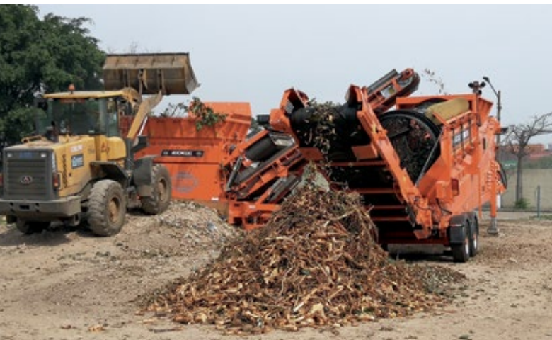
A powerful piece of kit: Shredding tropical timber requires a powerful shredder. As part of an FKKP project, this one was delivered to Rio de Janeiro with the support of Rio's partner city of Cologne. Since then it has been shredding green waste for further use and composting on a daily basis. © Ute Dreiocker, Stadt Köln
